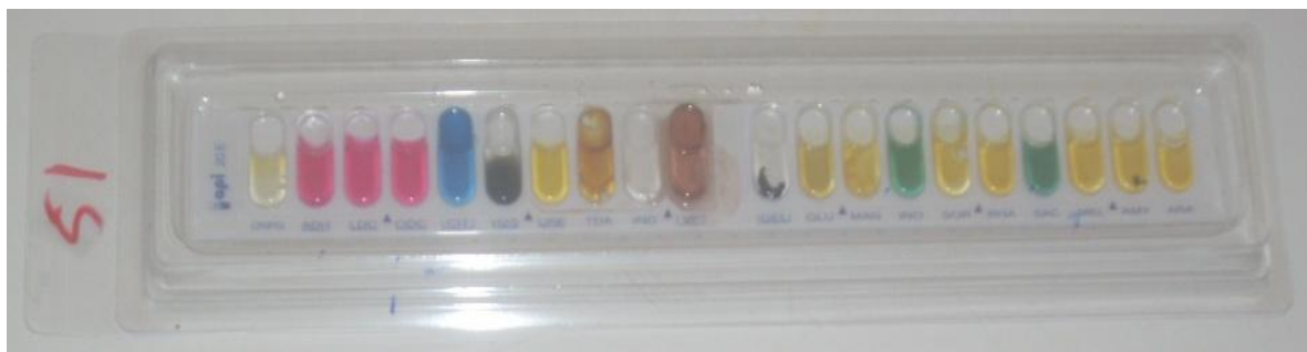
Plate 1: Typical Salmonella spp reaction of API 20E test kit with twenty reaction tests.
