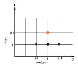
Figure 4.1: Computational molecule for the explicit numerical difference scheme.
