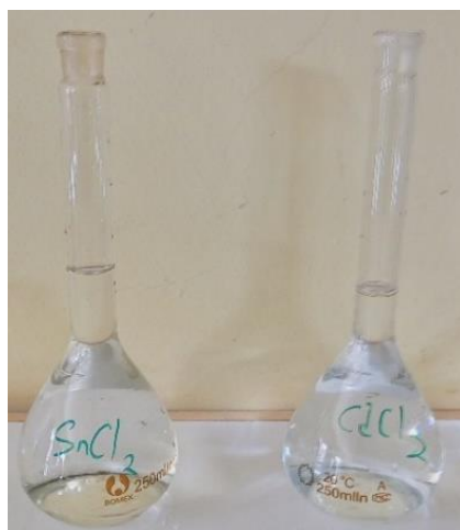
Figure 3.3: The prepared precursor solutions of cadmium chloride monohydrate and tin II chloride dihydrate
