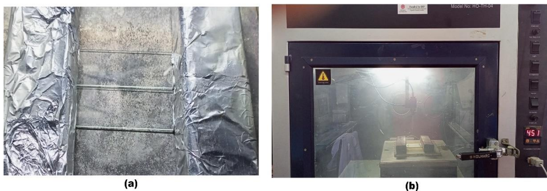
Figure 3.5: The process of depositing the thin films of cadmium-tin-oxide: (a) the clean microscope glass slides placed on top of the plate of the spray pyrolysis equipment. The slides are supported by iron tubes, each of length 15 cm, gauge 12. The tubes are wrapped in aluminium foil; and (b) the process of depositing the thin films at a temperature of 450 \pm 5 °C
