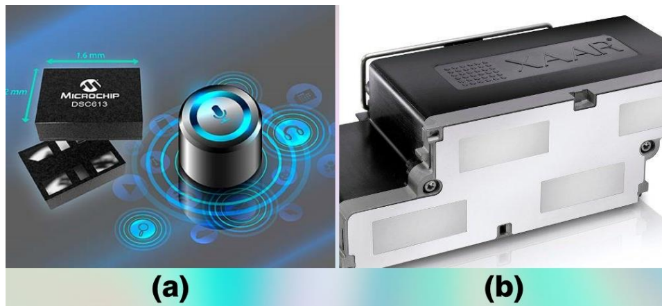
Figure 2.20: Some industrial applications of MEMS: (a) industry's multi-output Micro-Electromechanical Systems clock generator (image from: https://www.5gtechnologyworld.com/industrys-smallest-multi-output-mems-clock-generator/ . 06/11/2018), and (b) a Micro-Electromechanical Systems print head (image from: https://imieurope.com/inkjet-blog/2016/6/6/xaar-joins-the-si-mems-printhead-club . 06/06/2016)
